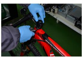
\*\* Turn the handlebars and place it in the correct position to ride, tighten the two small screws on the side with the Allen key on the multitool.
