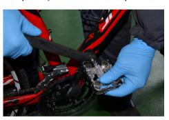
\*\*Be sure the pedal labeled "R goes on the right and pedal marked with "L" goes on the left side. In the hotel or hostel you'll find a wrench 15 that lets you tighten. (remember the pedals tighten or screw opposite of what you are accustomed to threading.
