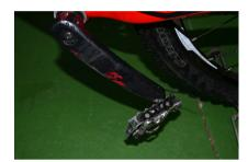
\*\* The pedals may be secured with cable ties to prevent loss during transport or in the saddlebags.
